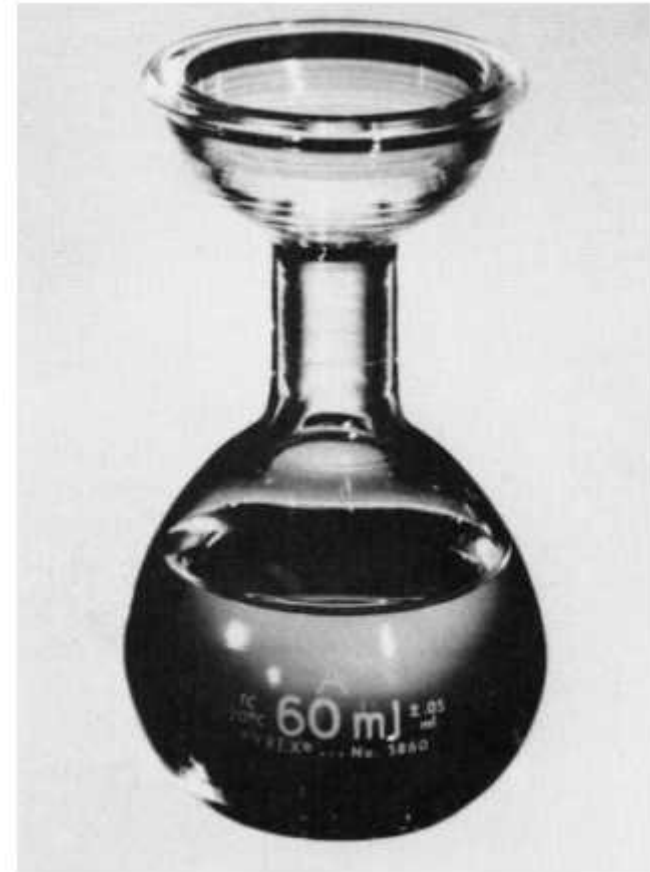
(c) 60 mL flask for collecting Saybolt sample
