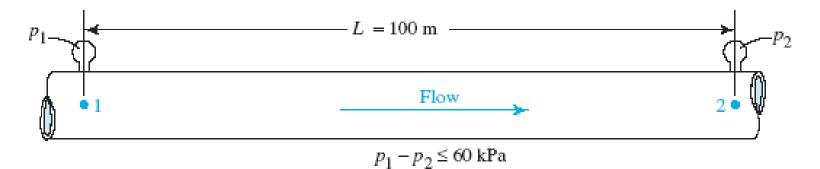
Step 1 Write the energy equation for the system. Step 2 Solve for the limiting energy loss . Step 3 Determine the following values for the system: Pipe flow diameter DRelative roughness D/ Length of pipe LKinematic viscosity of the fluid ; may require using  $V_{2000}$  Pul/
