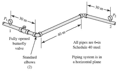
Initially, we ignore the minor losses and use Eq. (11–3) to compute a rough estimate of the allowable volume flow rate. This is accomplished in the upper part of the spreadsheet in Fig. 11.6 and it is identical to the solution shown in Fig. 11.5 for Example Problem 11.2. This is the starting point for Method II-B.
