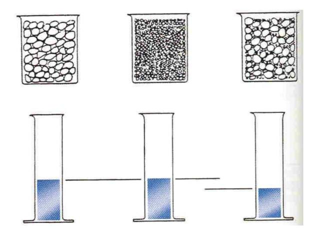
Amount of cement paste required in concrete is greater than the volume of voids between the aggregates.
